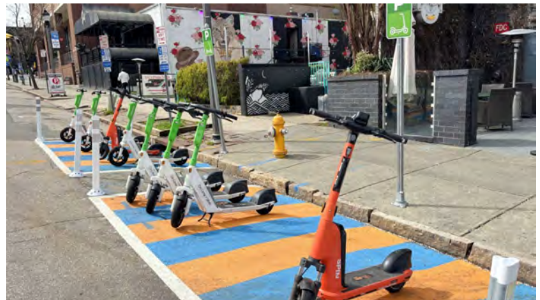
FIGURE 19: SHARED MICROMOBILITY CORRAL IN RALEIGH, NC Image source: City of Raleigh, NC
